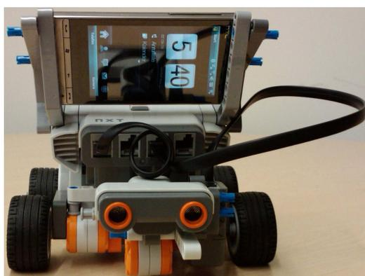
Figure 8.1: LEGO Mindstorms equipped with HTC PDA
