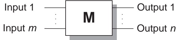
Figure 3.1: A generalized black-box software module M with m inputs and n outputs.
