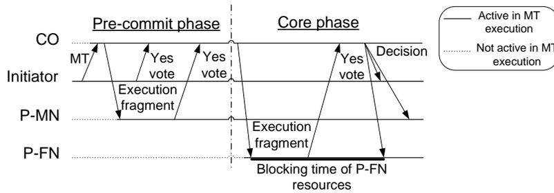
Fig. 5. Tolerating network disconnection – Decoupling concept
