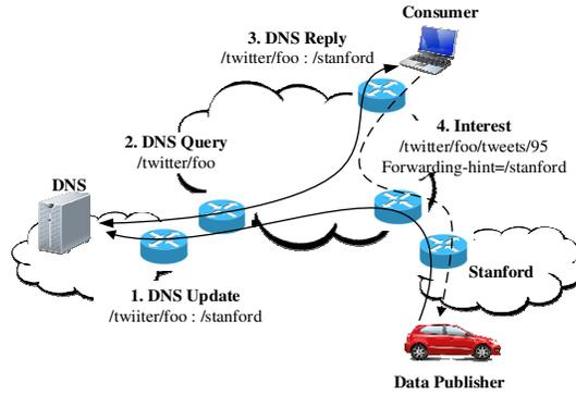
Fig. 24: DNS-Based Mapping for Data Fetching [161]
