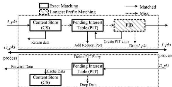
Fig. 7: Forwarding Process at NDN Node [6]
