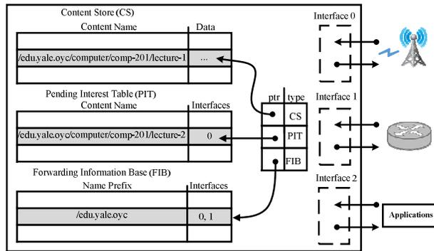
Fig. 6: NDN Node and its Forwarding Structures [10]
