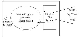
Figure. 3: Interface File System in a Smart Transducer.bylle
