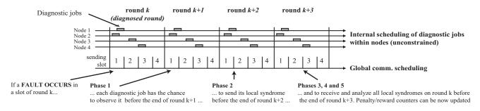
Figure 1: High level overview of the diagnostic protocol in a system with four nodes
