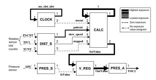
Figure 5. Exposure profile of target system
