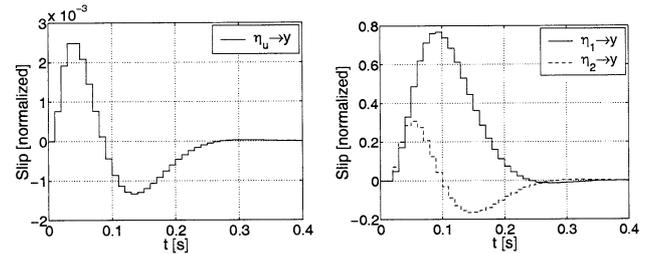
**Fig. 6** Output signal responses to impulse data errors in  $\eta_u$  (control signal),  $\eta_1$  (integrator) and  $\eta_2$  (observer). The plots have different scales.
