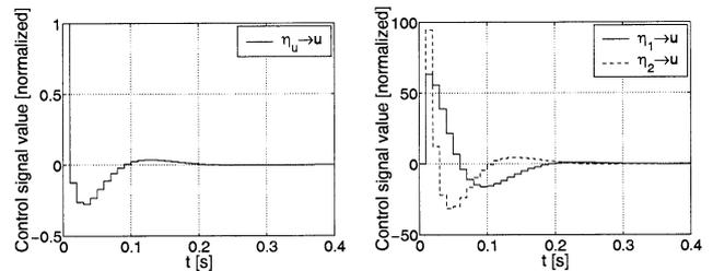
**Fig. 7** Control signal responses to impulse data errors in  $\eta_u$  (control signal),  $\eta_1$  (integrator) and  $\eta_2$  (observer). The plots have different scales.
