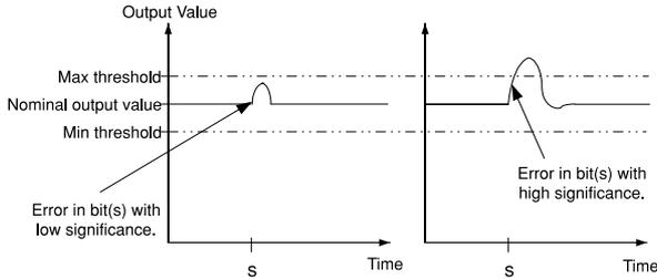
Fig. 1 Transient fault influence on the control error.
