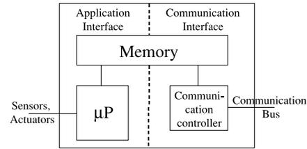
Fig. 2 A General architecture of a computer node.
