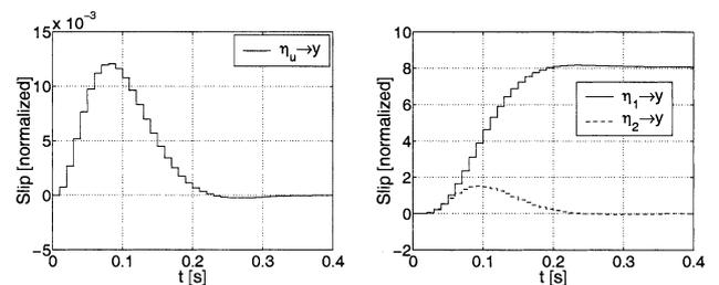
**Fig. 8** Output responses to step fault disturbances in  $\eta_u$  (control signal),  $\eta_1$  (integrator) and  $\eta_2$  (observer). The plots have different scales.
