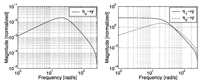
**Fig. 5** Sensitivity functions from  $\eta_u$  (control signal),  $\eta_1$  (integrator), and  $\eta_2$  (observer) to output,  $y$ . The plots have different scales.
