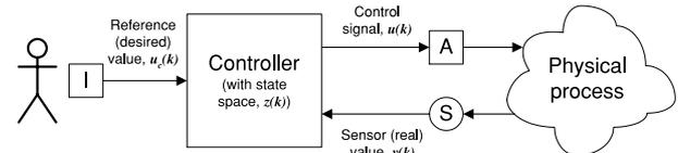
Fig. 3 General depiction of a controller and the corresponding physical process.
