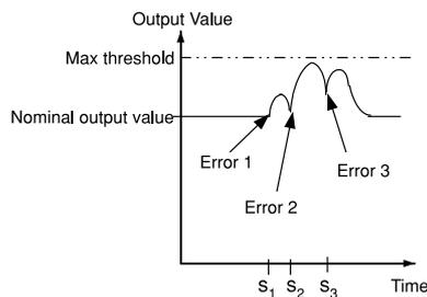
**Fig. 9** Simulations of the impact of three errors with different magnitudes occurring close in time.
