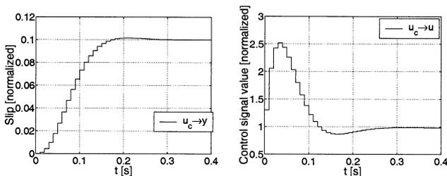
**Fig. 4** Step-input command-signal response of closed-loop system. The plots have different scales.
