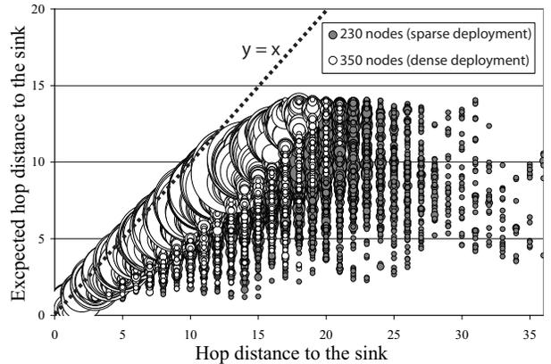
Fig. 1. Distribution of actual hop distances compared to expected distances. even the optimal spanning tree over such sparse network often results in a highly irregular topology.
